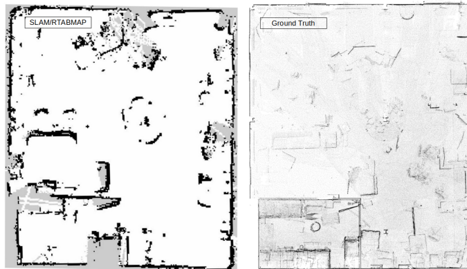
Fig. 8: Map analysis: The image on the right is the ground truth, and the image on the left is the computed map from RTABMAP SLAM
