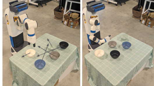
Fig. 1. An example of mobile robot tabletop rearrangement, where black arrows point to the desired rearrangement goals.
