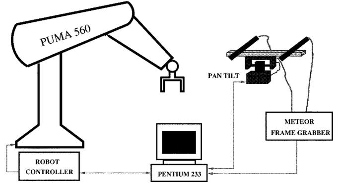
Fig. 5. Robotic workcell. In the present configuration, no specialized vision hardware was used.
