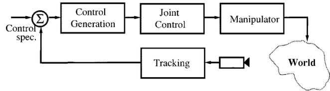
Fig. 1. The major components of a visual servo system.
