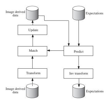
Figure 4: A module architecture which facilitates use of hierarchical control
