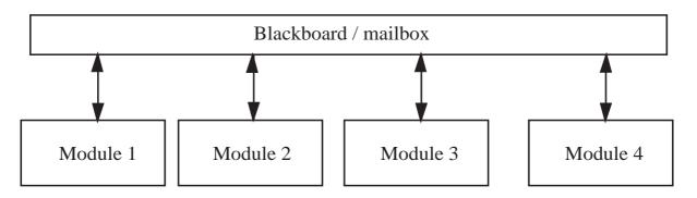
Figure 2: System architecture for heterarchical control
