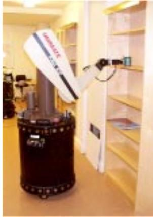
Fig. 3.: The XR4000 platform with a Puma560 manipulator.
