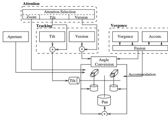
Fig. 5.: The modified cyclopean control architecture where the optical degrees of freedom and the pan motor have been added.
