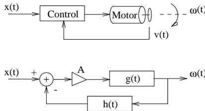
Fig. 2.: Example of standard control system for a DC-motor with tachometer feedback, with “normal” appearance at the top and the control schematic equivalent at the bottom. The driving signal from the controller to the motor is a voltage, proportional to the desired angular velocity. The tachometer readout is a voltage equivalent to the current angular velocity.
