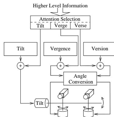
Fig. 4.: Overview of the proposed architecture for an equal eye dominance control scheme. Only the control of angular degrees of freedom have been shown.
