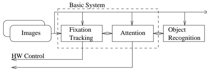
Fig. 1.: The basic system layout with a fixation - tracking module. This is followed by an overt attention module, enabling selection of interesting points or regions in the images. For the complete system an object recognizer is needed for supplying top-down information.
