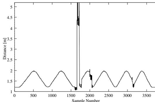
Fig. 6.: Fixation distance for the combined disparity and accommodation control. Normal operation is based solely on disparity, but when no disparity match can be obtained the accommodation process is activated. The objects moves towards and away from the object between 1.2 and 2.1m.
