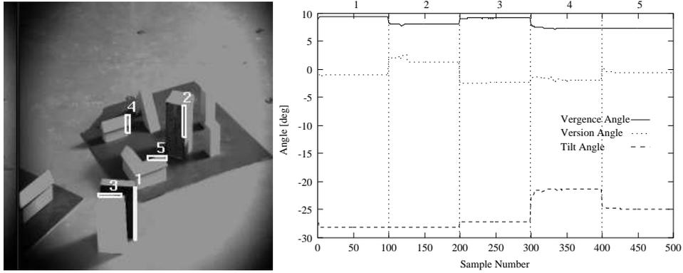
Fig. 7: **Left:** The receptive fields (white) on top of the input image. The numbers denote the rank in which they were selected, with number 1 as the most salient region. **Right:** shows the Vergence, Version and Tilt angles during fixation shift. Shifts occur at sample 0,100,200,300 and 400.
