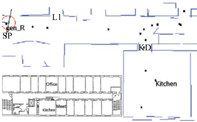
Fig. 3. The part of the lab environment (schematic drawing in the left lower corner) traveled by the robot together with one guiding person. The black dots without label mark the positions where the system decided to generate a new (hypothesized) region. The labeled dots refer to an explicitly specified region's center (Kitchen) and the starting point (gen.R). Already stored regions were not considered – each dot marks a point where the previously accepted representation does not match the current (hypothesized) one sufficiently anymore. A movement threshold of one meter was assumed, the similarity distance threshold was set to 1.5, changes were accepted immediately.
