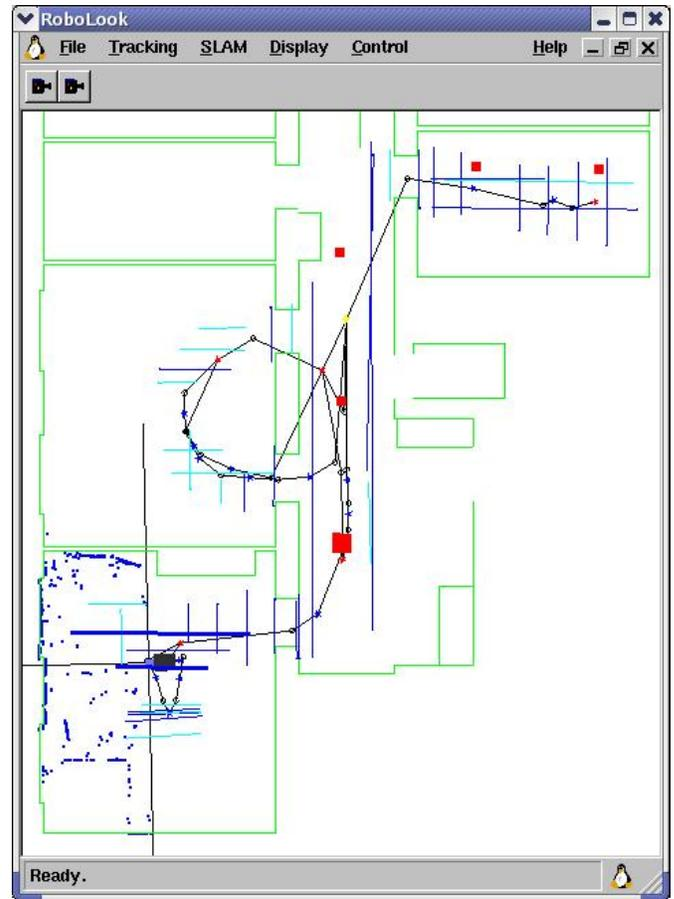
Fig. 6. This is the map obtained using only the vision features. The walls of the building are shown for reference. The final graph has 78 pose, 49 feature and 25 star nodes. 3,377 pose nodes were eliminated by graph reduction which also formed 3 loops. It took 2.5 times as long as the EKF.
