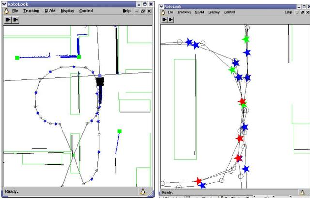
Fig. 8. Here we see that two star nodes have been combined when closing the small loop. We can see a 4-pose star. We can also see the inclusion of a corner point between two walls found using the laser. The final topology of the graph becomes rather intricate upon returning to this region two more times. One sees that stars near each other but with the robot facing the opposite direction were not combined.
