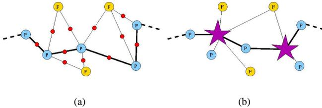
Fig. 2. Introduction of a star node. a) initial state, b) Star nodes are introduced in the graph between every other pose node. The stars are connected to all state nodes that the energy nodes it replaced were connected to.
