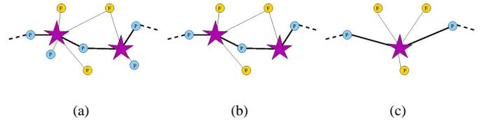
Fig. 3. Graph reduction. a) Initial state of graph from Figure 2. b) Pose nodes connected to only one star node can be reduced. c) Two star nodes of level  $l$  can be combined into one star nodes of level  $l+1$ .
