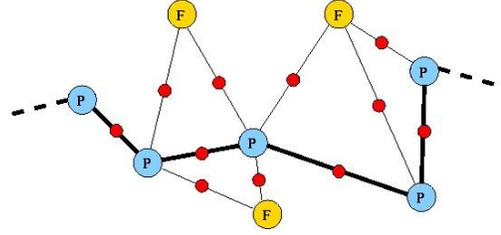
Fig. 1. Small part of a graph. The red/darker nodes are energy nodes. These can be either odometry nodes or measurement nodes. The measurement nodes connect a pose node with a certain feature node i.e. the data association. The lighter nodes are state nodes, where **P** denotes pose nodes and **F** feature nodes.
