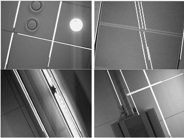
Fig. 5. Snapshots of the ceiling along the path showing the line detection output.
