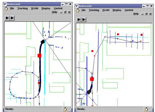
Fig. 7. Here it is shown how the tail needs to be left long while the long line on the ceiling is still accumulating dense information (moving up). As soon as the line become 3 dimensional the tail can be reduced and the entire path can use the full 3-D feature (moving down).
