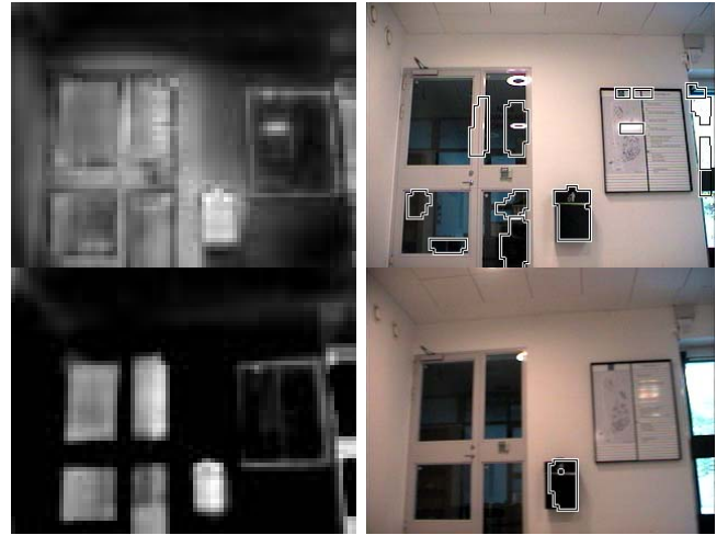
Fig. 4. Saliency maps (top, left: S_{bu} , bottom, left: S_{id} ) and MSRs in a loop closing example: Top: scene at beginning of sequence. Bottom: revisited scene, 592 frames later, searching for the black waste bin with top-down attention.
