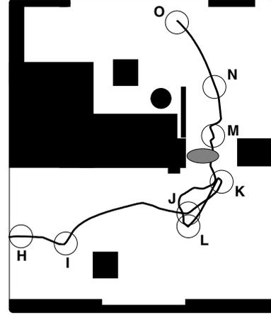
**Figure 7:** The trajectory of the robot from the corridor (H) to a goal point in a room (O). The grey ellipse denotes a person that was leaving the room, when the robot was at location K. The situations labelled by the symbols H-O are explained in the text. The circles at these points depict the size of the robot.
