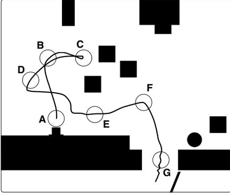
**Figure 5:** The trajectory of the robot starting at the charging station (A) and leaving the room towards the corridor (G). The black obstacles denote chairs, two shelves, a table and a waste bin. The situations labelled by the symbols A-G are explained in the text. The circles at these points depict the size of the robot.
