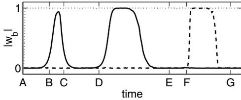
**Figure 6:** Time plot of the absolute values of the weights:  $|w_{obst}|$  (dotted curve),  $|w_{goto}|$  (solid curve), and  $|w_{door}|$  (dashed curve) (see equation 10). The time instances labeled by the symbols A-G correspond to the situations in Figure 5.
