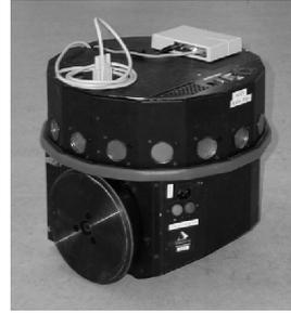
Figure 2: The Scout robot used in the experiments.
