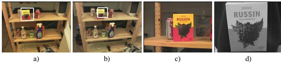
**Fig. 4.** a) and b) Images observed by the left and right head camera, respectively. The windows show the position of the raisins package estimated by the recognition system. c) image observed by the eye–in–hand camera, and d) destination image used for 2 1/2 D visual servoing.
