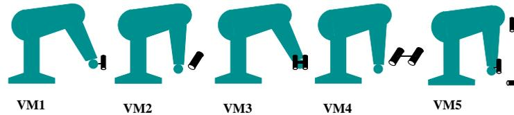
**Fig. 2.** Most common camera–robot configurations: monocular eye–in–hand, monocular stand–alone, binocular eye–in–hand, binocular stand–alone and redundant camera system. In our system, we are using a combination of VM1 and VM4 which is a special case of VM5.
