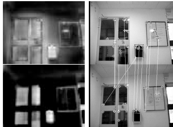
Figure 2. Loop closing example: top: scene at beginning of sequence. Bottom: revisited scene, 592 frames later, searching for the black waste bin with top-down attention. Left: saliency maps S_{bu} (top) and S_{td} (bottom). Right: the most salient ROI (top) and its redetection with top-down attention (bottom) as well as the matching of all Harris points. In our approach, we use only the points inside the ROIs what reduces the complexity strongly and eliminates false matches.
