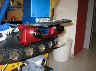
Fig. 1. Left: The experimental platform, the PowerBot Dumbo from ActivMedia. Right: A close up of the Videre stereo rig used in the experiments.
