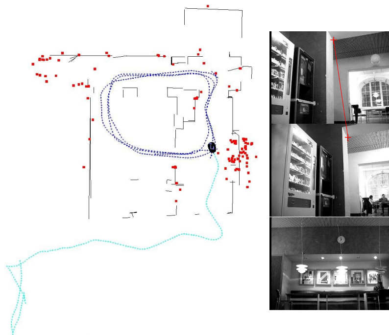
Fig. 1.5. The SLAM map is shown as red squares at the locations of landmarks. To help visualize the environment, a separately made laser scanner map is superimposed on this map. Also shown are the trajectories from when the map was built (3 loops) and when the robot was trying to localize. The feature match between the evening database image image (top) and the daytime localization experiment (middle) is indicated. The bottom image corresponds to the area of the map where the density of landmarks is greatest.
