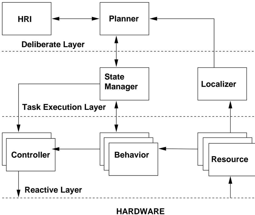
Figure 4: Architecture for the service robot systems
